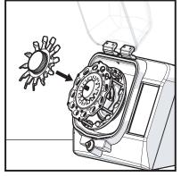
**3.** Place the 15 mL Tube carriage and 15 mL Finger Plate on the Bead Ruptor Elite<sup>™</sup> Hub.
