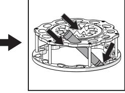
**2.** Ensure that tubes are loaded as shown and seated properly in the tube carriage.
